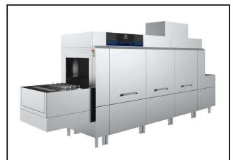
520731 (EFTD052EL1U1M5L385AU) Flight type Dishwasher, 1 tank, 5200 dishes/h, electric, 750mm loading, 1000mm unloading, 55mm conveyor, left to right
